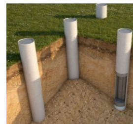
Figura 2.10 - Estacas de betão armado. [ https://dluxeinternacional.com/wp-content/uploads/2017/11/Pile-Concrete-types-of-pile-foundation.jpg ]
