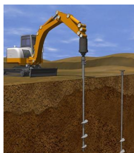
Figura 2.9 - Estacas Helicoidais. [ https://cdn.shopify.com/s/files/1/1887/6189/collections/Screw_Piles.jpg?v=1490856044 ]
